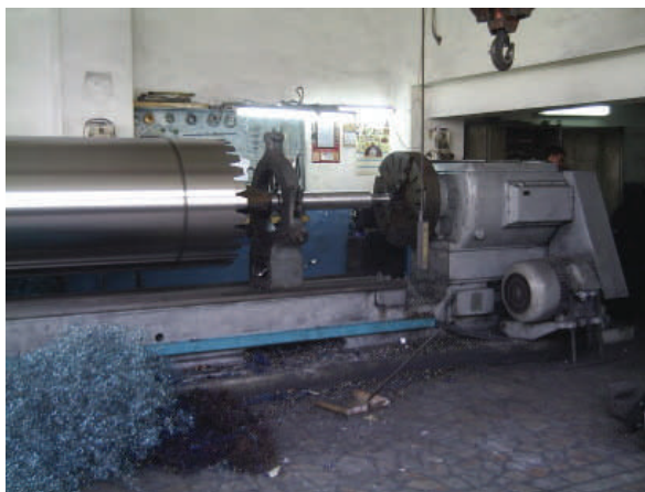
The Lathe Showing the Motor and the Turned Steel Drum
