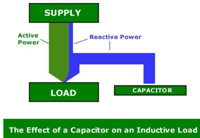
This reduces the burden on the supply for a given load, and is usually the source of most beneficial effects associated with power factor correction.
