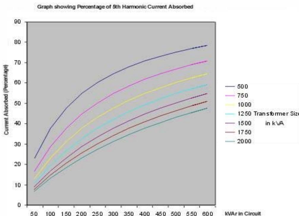
For example, the connection of a capacitor bank of 200kVAr to a low voltage network fed from a typical 1000 kVA transformer would have the effect of absorbing approx. 37% of the 5<sup>th</sup> harmonic current produced by the load.
