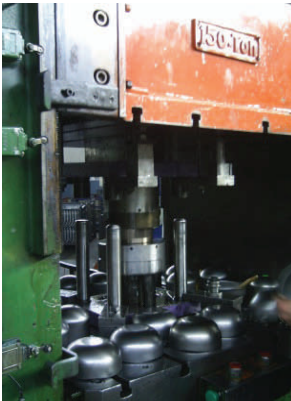
The Press Tooling Showing the Formed Components
