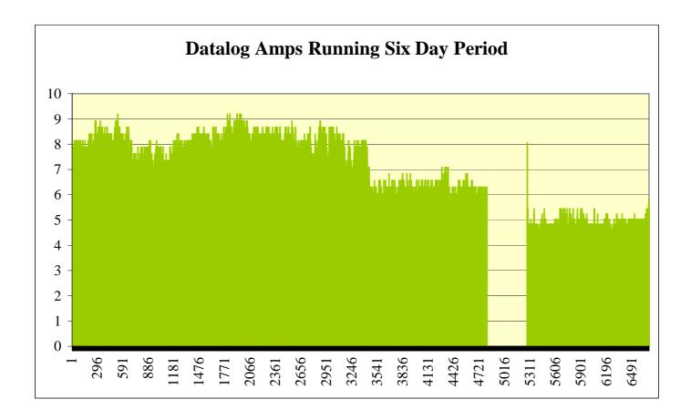
The break at data point 4760 is the Sunday when the machine shop was closed. The EnviroStart was switched into optimisation at data point 3387 and demonstrated a shift in mean current consumption of 8.2A to 6.3A. This gives a paid kW saving of >24% overall.
